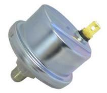
PTR transducers require a good earth connection via their threads, so **DO NOT** use any PTFE tape or other sealant on the threads.
